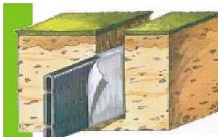
Fig 6 - Interceptor Curtain Drain
