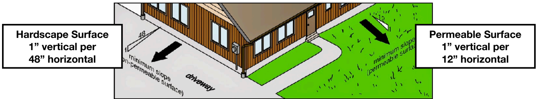
Fig 1 - Drainage Slope Relative To The Structure
