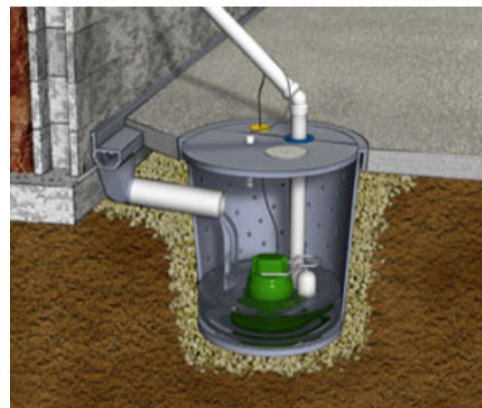
Fig 4 - Exterior Sump Pump
