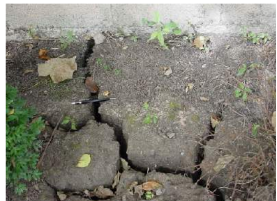
Fig 4 - Visual Appearance of Expansive Soils When Dry
