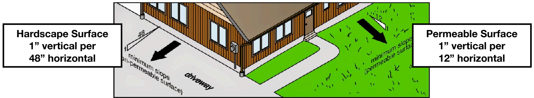
Fig 1 - Drainage Slope Relative To The Structure
