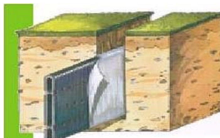
Fig 6 - Interceptor Curtain Drain
