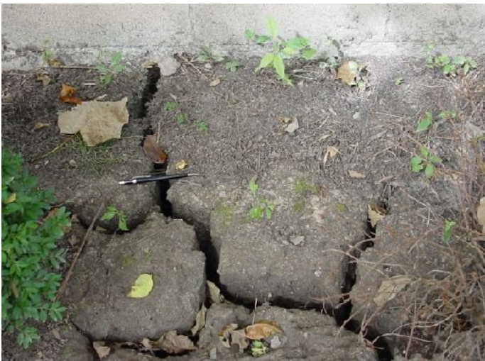
Fig 4 - Visual Appearance of Expansive Soils When Dry
